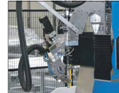
3 or 5 axes cutting heads
