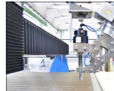
Static or conveyor belt worktop
