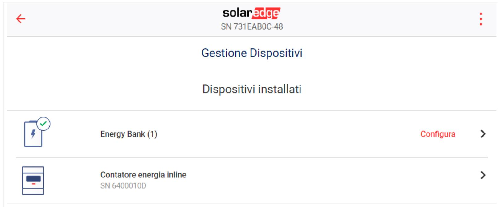
The screenshot displays the 'Gestione Dispositivi' (Device Management) screen in the SolarEdge Energy Net app. At the top, the 'solar<sup>edge</sup>' logo and the system ID 'SN 731EAB0C-48' are visible. Below the title, the section 'Dispositivi installati' (Installed Devices) lists two items:
