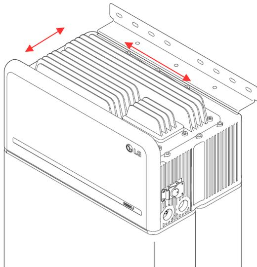
16. Assemble Standing Bracket #2 (flat) using six (6) M6 bolts to fix the pack onto the wall
