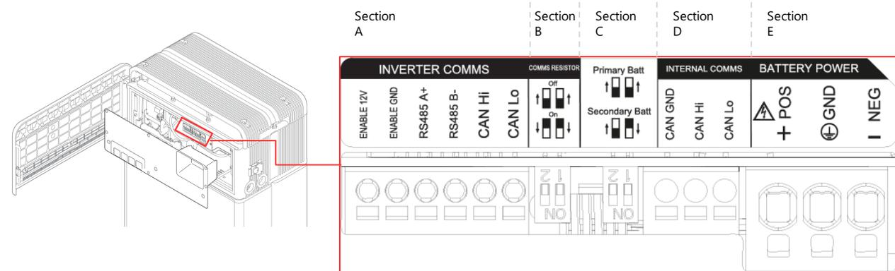
**Section A:** Inverter communication ports including CAN/RS485 and enable lines
