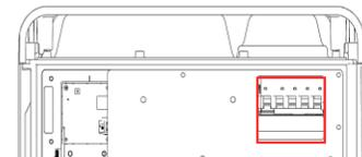
Turn on the circuit breaker switch and close the front cover
