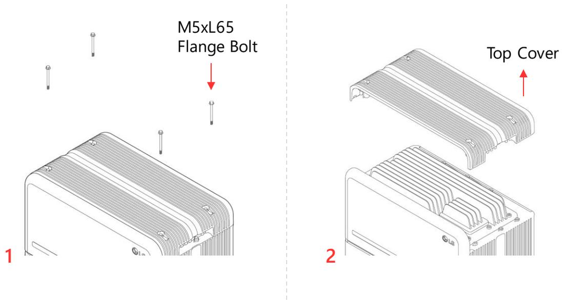
14. Tighten six (6) long flange bolts with a torque of 5N.m
