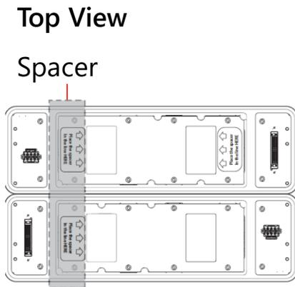
8. Place the Battery Control Unit on top of the spacers, and align with the Battery Module
