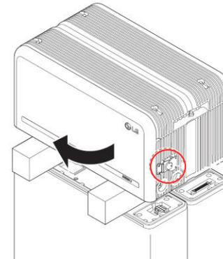
Hold and turn the handle counterclockwise to open the front cover
