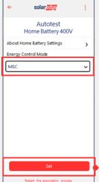
Set the battery operation mode to Maximum Self Consumption (MSC). Then check from the status section that the batteries have started working.
