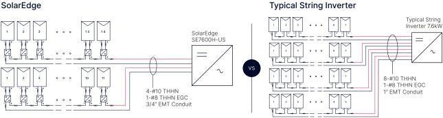
Cost of a 60' home run from the PV array: \$169.20 Only two strings required for a 25-panel system
